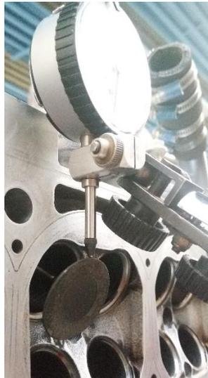
Figure 22: Jeu radial des soupapes
